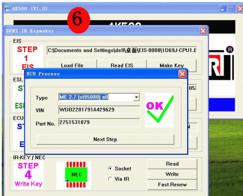
4. With "Next Step" function of the ECU to generate new data and functions with EEPROM to write back.
