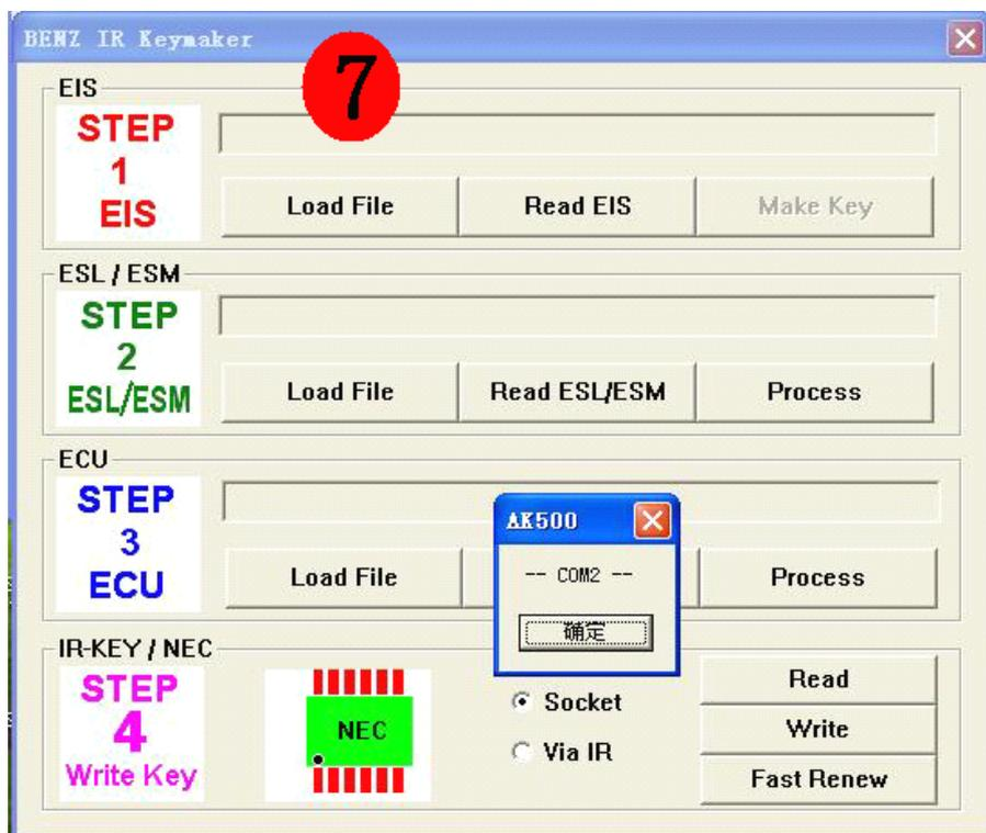
3. Select "COM2", after using "Load, BIN" the Key to open the need to write data, and "Programming" to write the new key (Figure 8).
