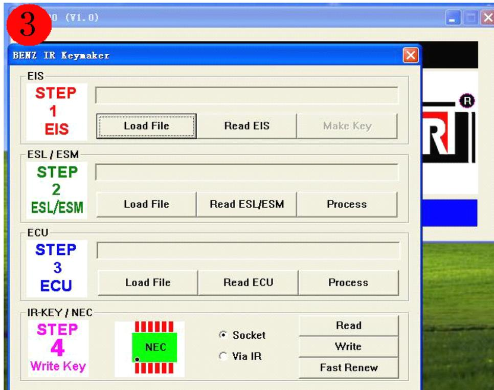
2. With "Make key" function, open the "EIS Process", we can see EIS information, Key end-of-life status and the use of the state, in the "New key" column to choose the key number needs to be done, and "Generate EIS new file + Generate new key file" (to generate new data and the key to the EIS data) to deal with function keys, the software automatically generates the new data as well as the Key of EIS data and stored in the original directory (Figure 4);
